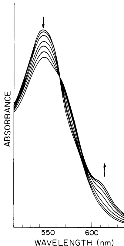
Figure 3. Spectral changes occurring upon titration of a 1.0 \times 10^{-4} M toluene solution of Fe(HmCap) with 0.0884 M 1,2-Me 2 lm in toluene at 23.1 °C. The final base concentration is 4.6 \times 10^{-3} M.
